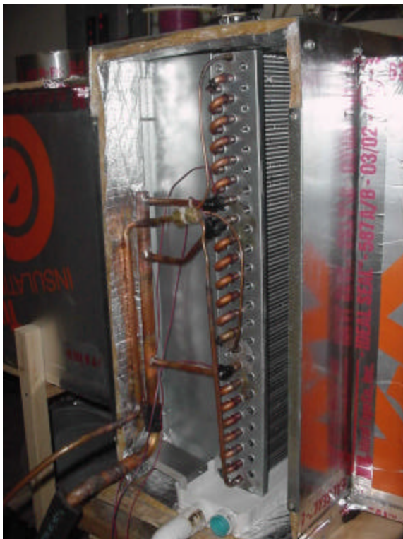
Coil refrigerant distribution (3 circuits)
