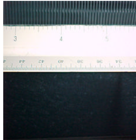
15.5 fpi, lanced sine wave fin
