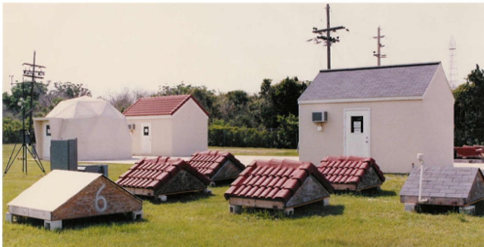
Figure 10. Small scale roof models to test roof coverings
