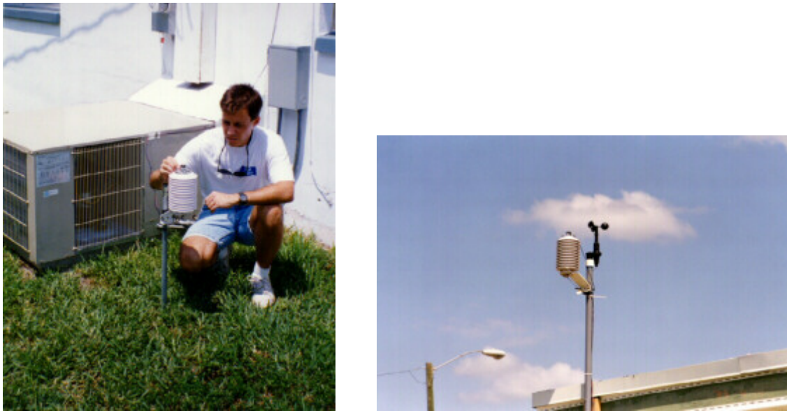
Figure 2. FSEC research engineer, Jeff Sonne, adjusts a pyranometer leveling base on the apparatus used in the measurement of condenser air and insolation conditions at site 2 (left). Example of a roof top meteorological station (right).
