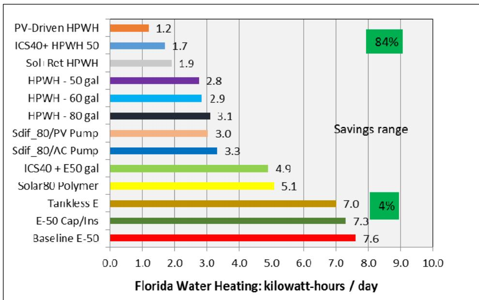
**Figure 7: Representation of various electric water heating systems daily electric use compared to a baseline (standard 189 L electric) and the potential for energy savings (4%-84%)<sup>3</sup>**
