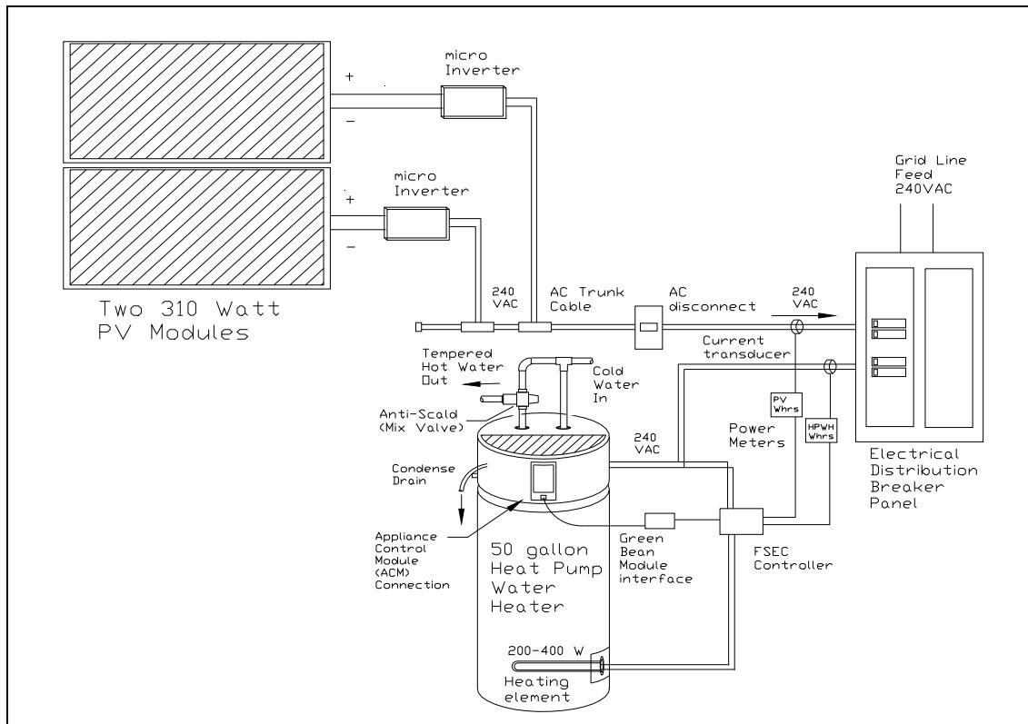
**Figure 2: Schematic diagram of prototype PV-assisted HPWH.**
