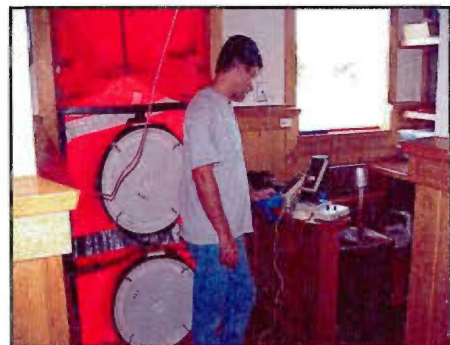
Figure 24. Blower door set-up installed in pick-up doorway.
