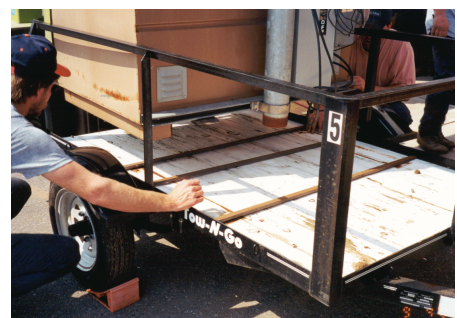
Figure 11 Temporary floor fix
