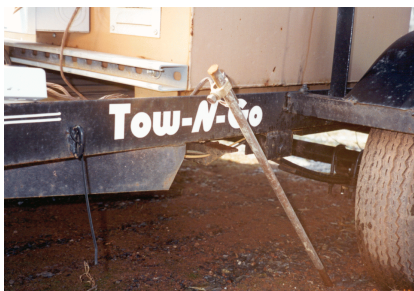
Figure 10 Floor brace breaking away
