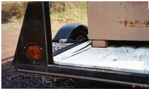
Figure 8 Enclosure sinking into wooden floor
