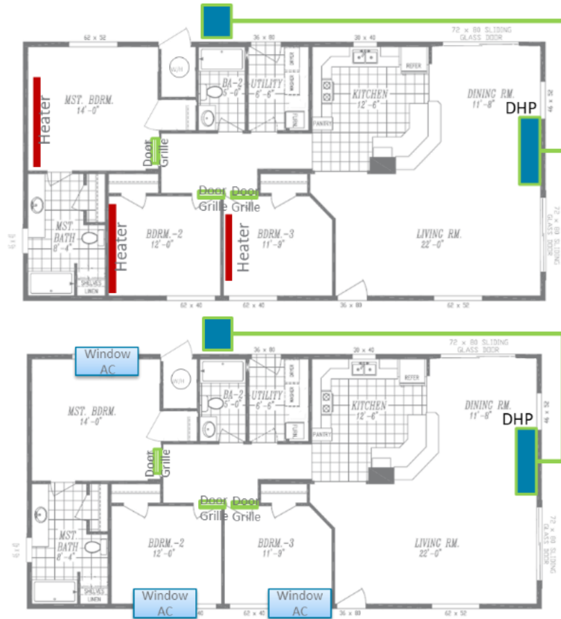
Figure 2a. Zonal Heating Lab Homes setup; Figure 2b. Zonal Cooling Lab Homes setup. Source: PNNL 2020.
