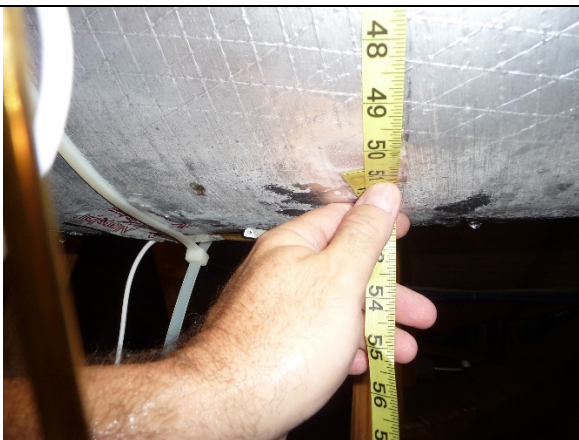
Figure 20. Example photo of jacket circumference measurement made on main trunk T2. Light condensation was on sides and larger water droplets on bottom of jacket (9/18/20).
