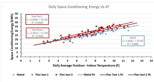
Figure 2. Daily cooling energy use of Tests 1 and 2.
