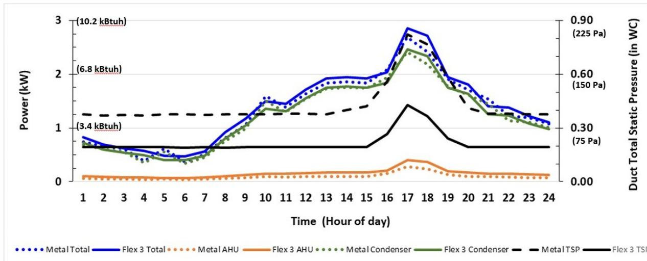
Figure 4. Cooling power use and fan TESP measured in two systems simultaneously during a typical summer day.
