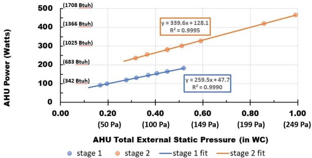
Figure 5. AHU ECM measured power versus TESP shown at first and second stages of cooling operation.
