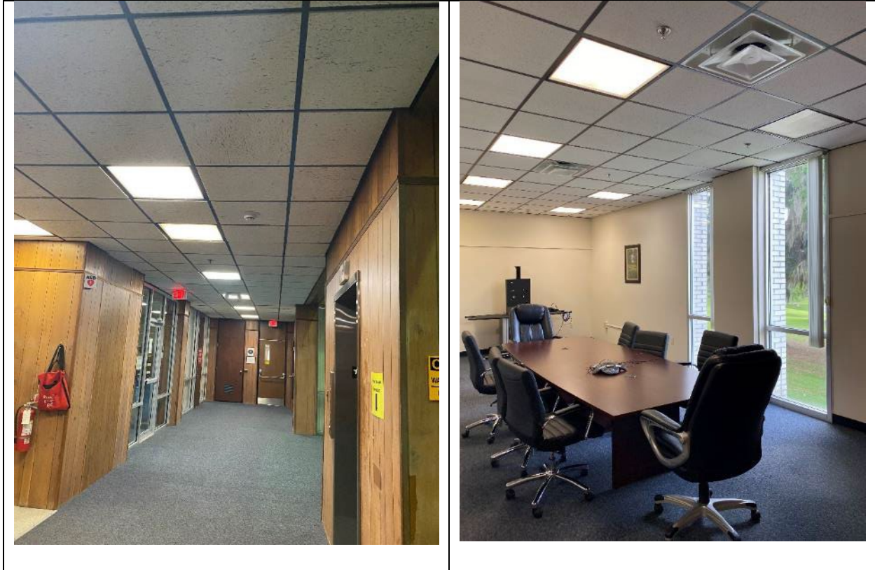
Figure 28. Right: Open areas and corridors under T8 “U” 32 watt lamp fixtures typical throughout building; Left: Desktop illumination in east conference room with natural sidelighting was more than adequate. This is a good application for occupancy and light dimming control.
