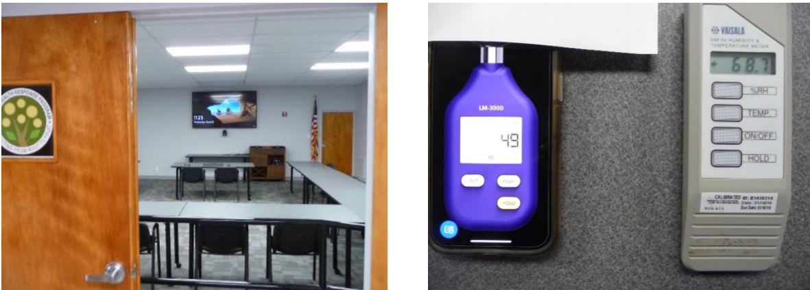
Figure 4. Left: Partial view into the east conference room with new LED lights and occupancy controls. Right: Desktop illumination in east conference room varied from 46 fc to 71 fc, however the space was overcooled to about 69° F while unoccupied.
