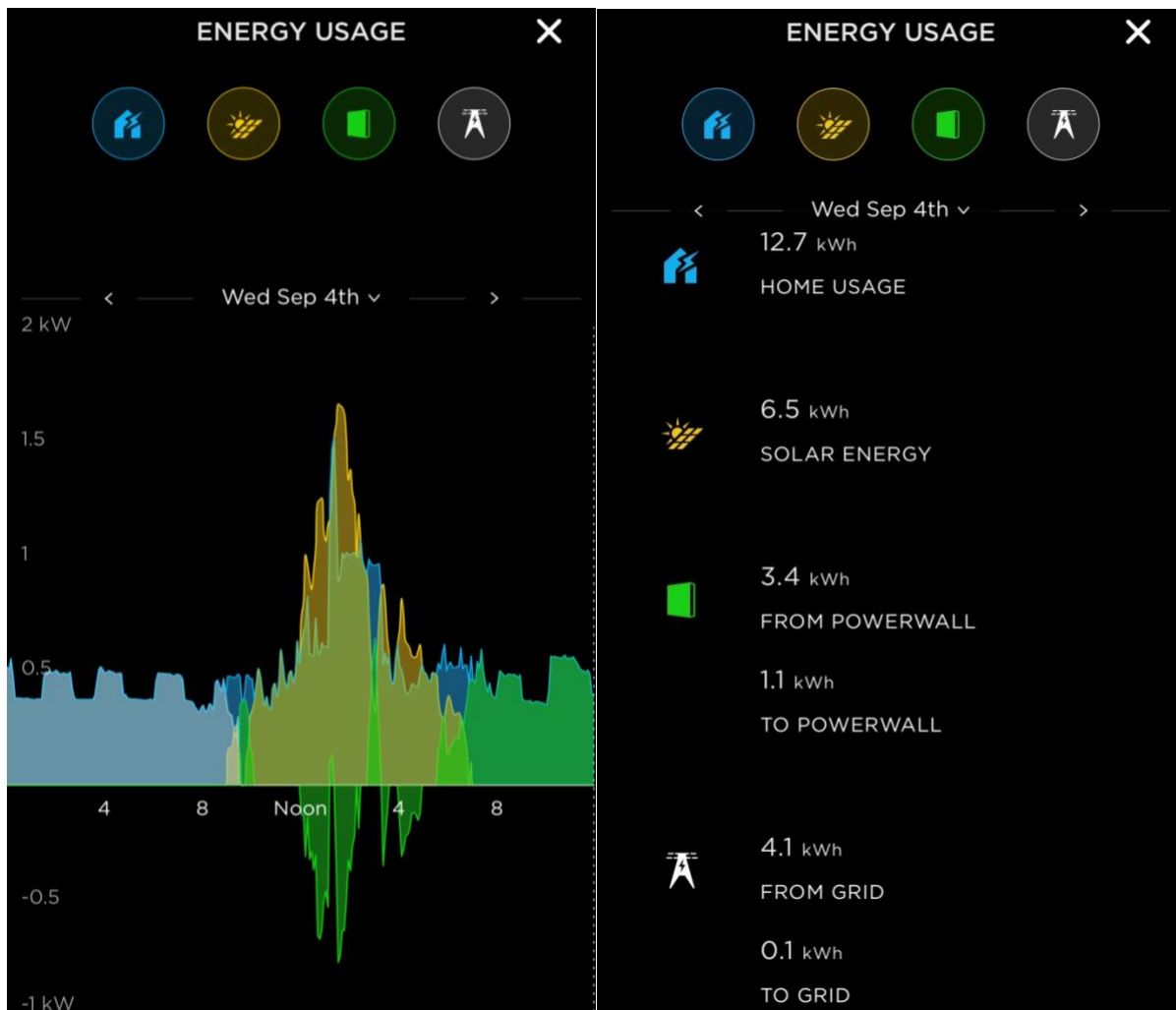
Figure 14: 4 Sept. 2019: Performance of solar & Powerwall system during Hurricane Dorian. Closest approach at 4 AM
