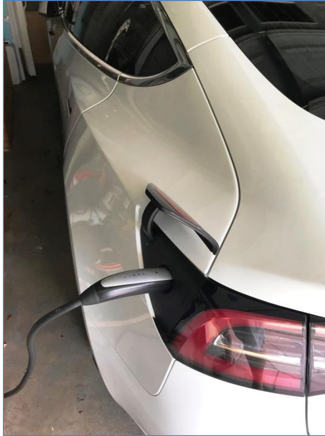
Figure 17: Using a Level 1 charger with solar the day after Hurricane Dorian to add range to a Tesla Model 3
