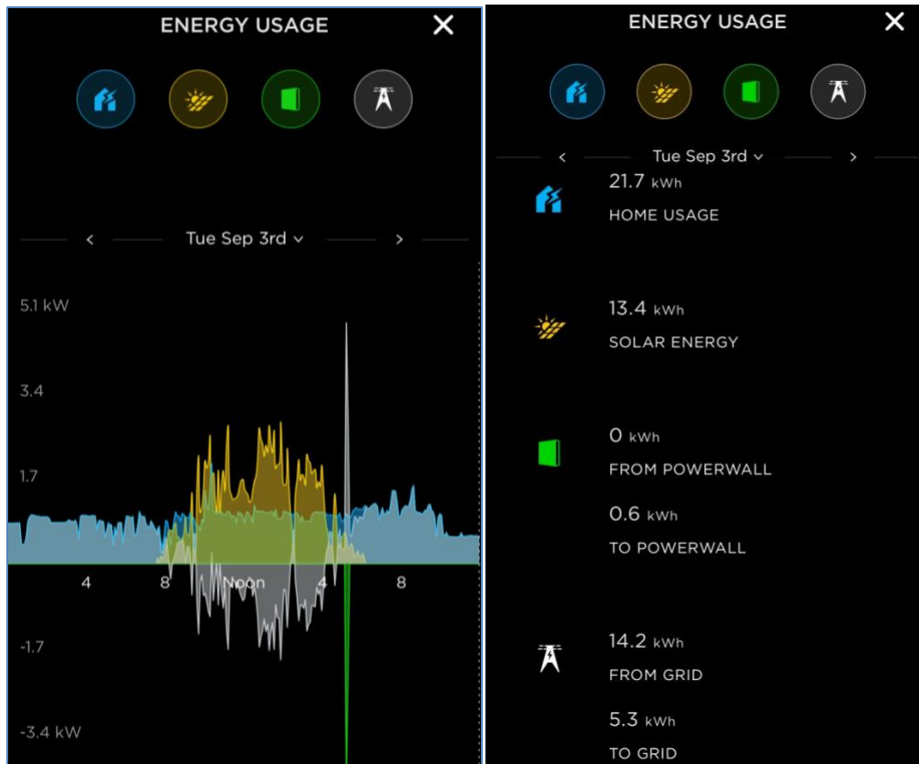
Figure 11: Performance of solar, grid, storage and home energy systems on 3 September as hurricane approached
